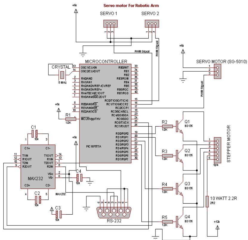
Figure 9: Electric Schematic Diagram of the Control Board
