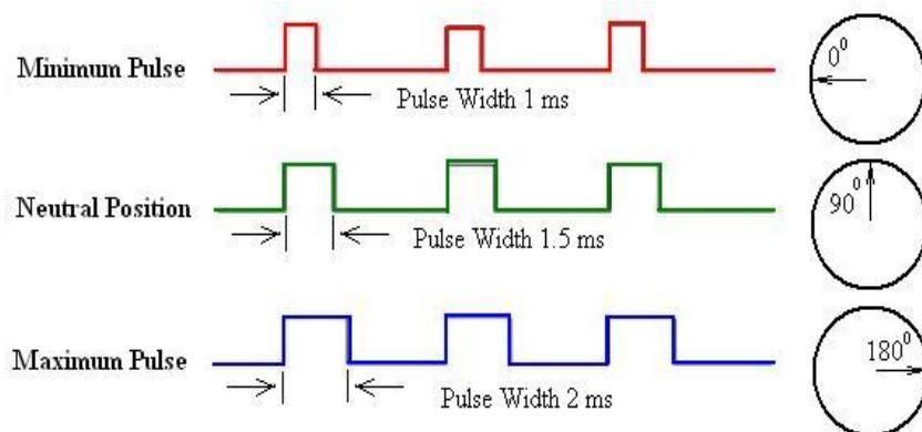
**Figure 5: PWM Signal for Servo Motor Position Control**
