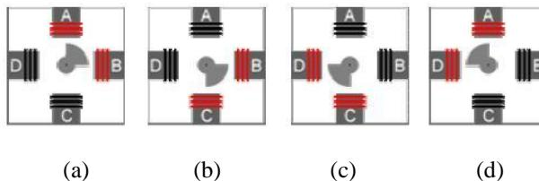
**Figure 3: Basic Principal Operation of Stepper Motor**
