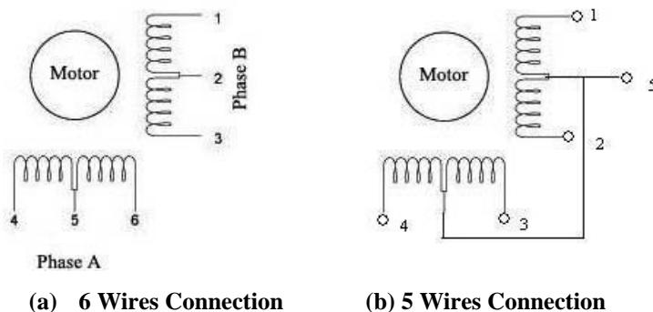
**Figure 2: Example of Various Stepper Motor Wire Configuration**
