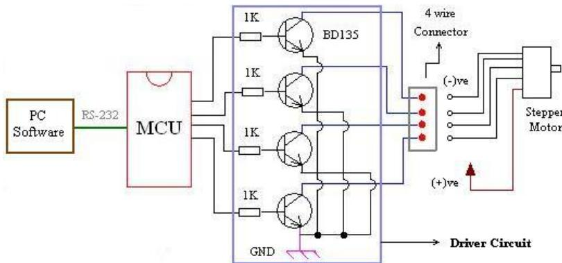
**Figure 4: Stepper Motor Driver Circuit for 5 Wires**
