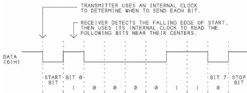
**Figure 10: Basic Asynchronous Data Transmission System [9]**
