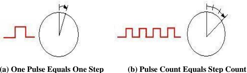
**Figure 6: Stepper Motor Rotation System Based on Pulses**
